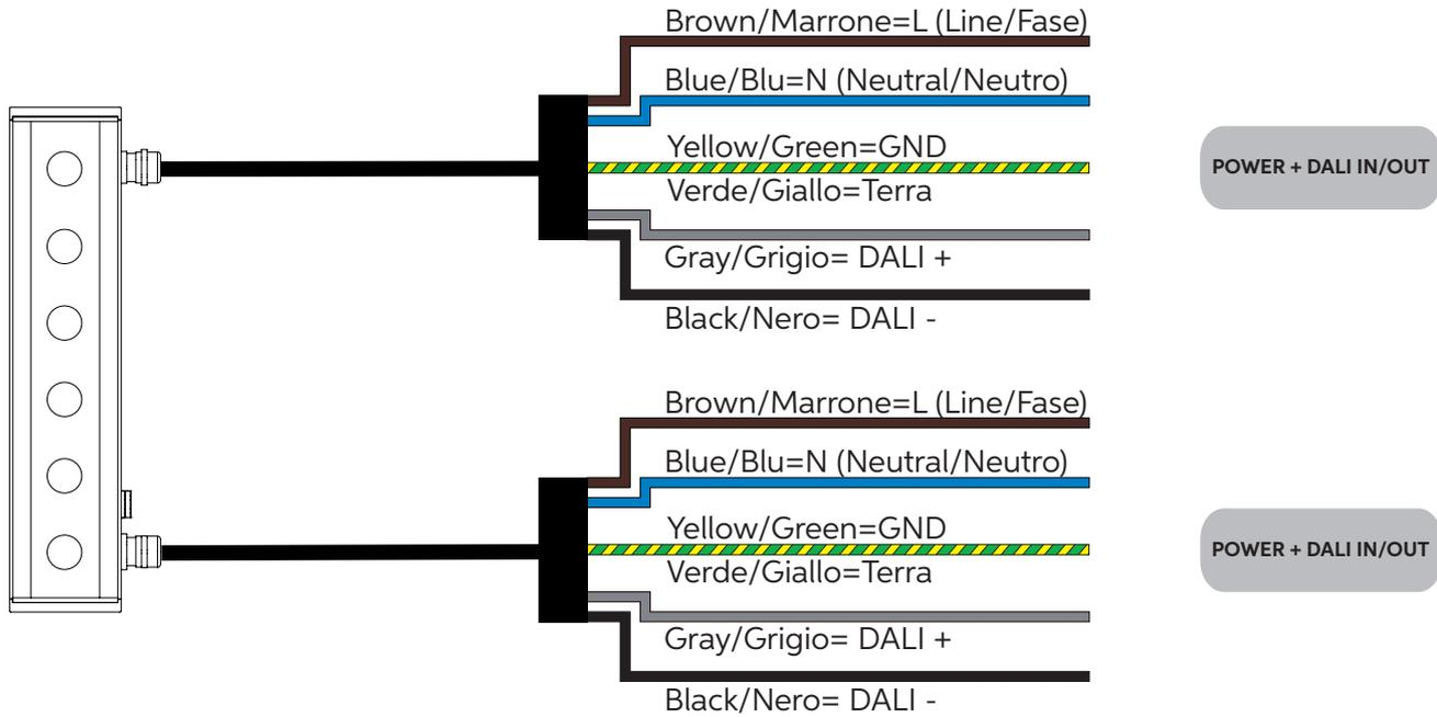
**Note:** in absence of DALI signal the LEDs will remain ON.
